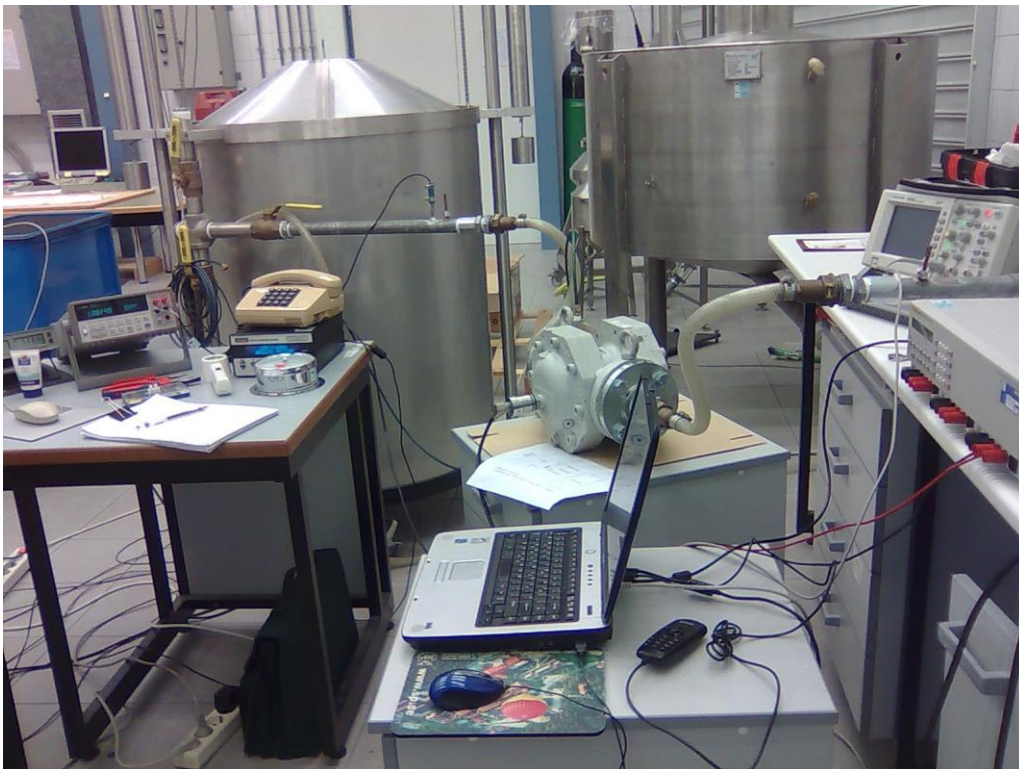
Figure 1. Partial view (1) of the experimental arrangement with Bell Prover reference facility.
