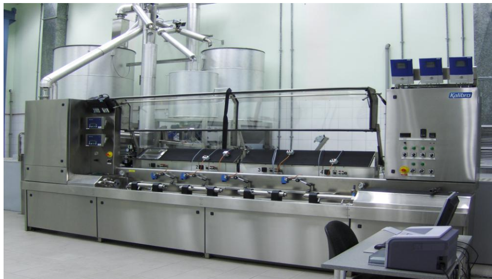
Figure 1. Overview of VEMIT Kalibro water flow test facility
